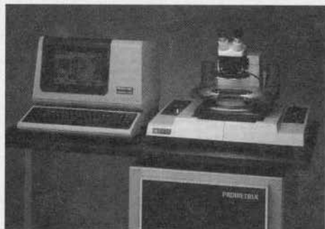
LithoMap LM20 Lithography Characterization System
