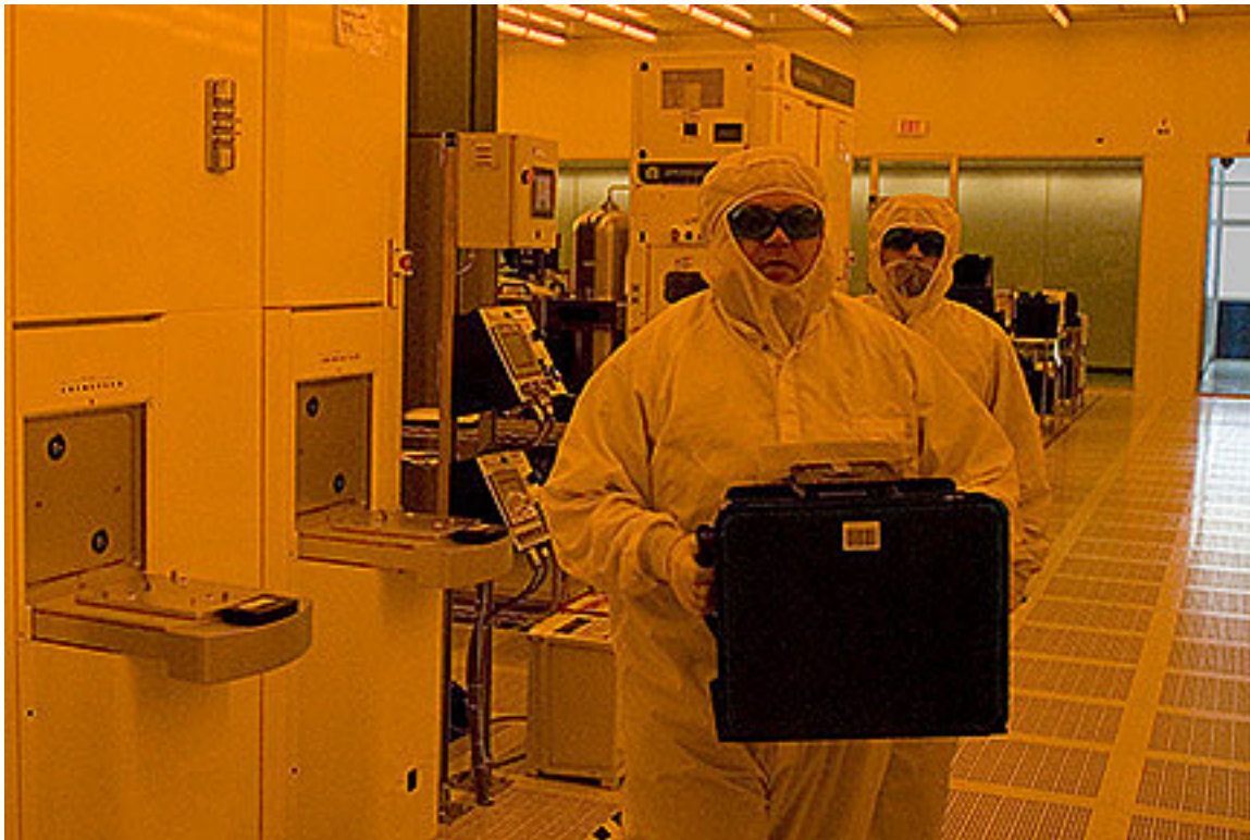
Inside Albany Nanotech: A worker lugs a 300mm FOUP to its next station. The yellow lighting tells you it is the lithography bay. Even though today's photo-resists are no longer sensitive to visible light, old traditions die hard anywhere where this is manufacturing intent. AlbnyNT_0703_011
