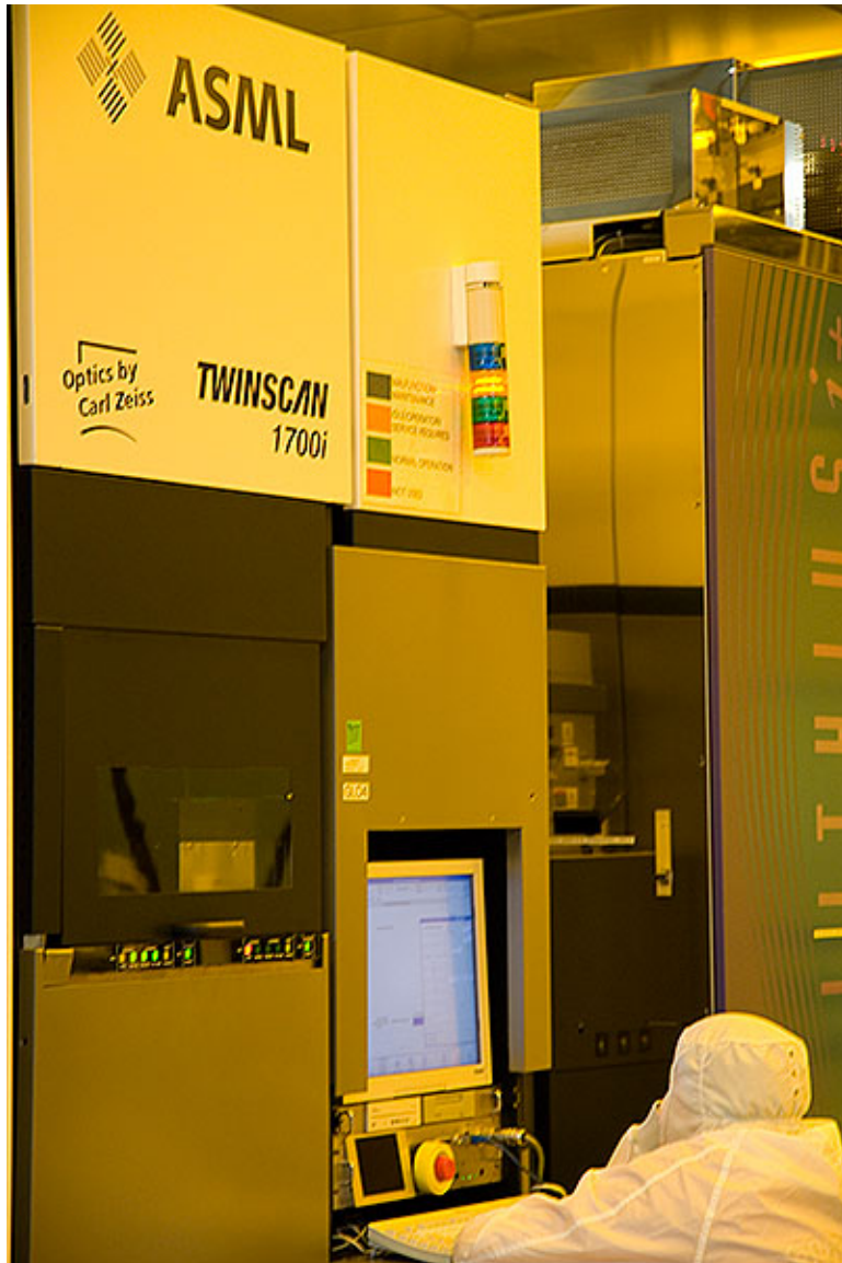
IBM's 323 facility: Too Cool for School Tool — the cutting edge of manufacturing lithography: Hyper-NA immersion IBM323_0703_012
