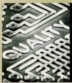
Applied Materials AME 8100 Series Plasma Etch System etched the symbolic word "QUALITY" into the plasma oxide layer of a semiconductor chip with VLSI precision not possible before. Scanning Electron Microscope (SEM) photograph is 1,400 times actual size. The etch is approximately two microns deep with line-widths as narrow as one micron or 1/25,000th of an inch.
